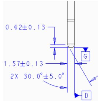
Figure 69: SFF Primary Connector Gold Finger - Detail D
