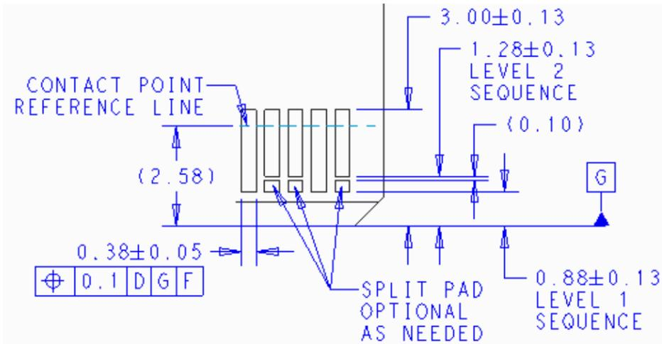
Figure 70: LFF Gold Finger Dimensions – x32 – Top Side (“B” Pins)
