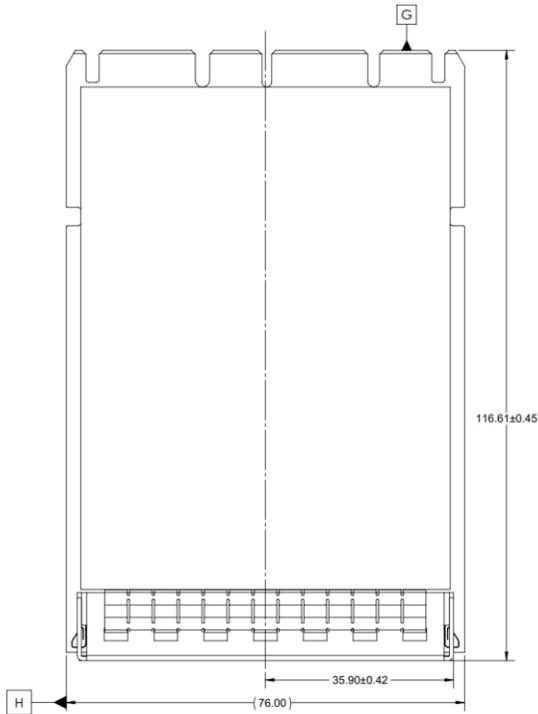
Figure 47: SFF OCP NIC 3.0 Card with Internal Lock CTF Dimensions (Front View)
