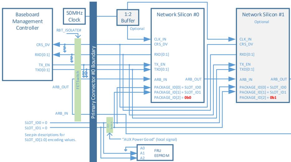
**Note 3:** The baseboard implementation shall maintain the arbitration ring integrity when there exists one or more cards that are not present, plugged in but are powered off, or in ID Mode.
