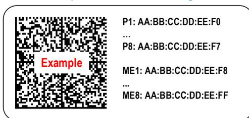
Figure 66 illustrates the use of ellipses in the human readable text to individually indicate a range of Port and Management MAC addresses. In this example, the 2D data matrix shall contain all 16 MAC addresses.
