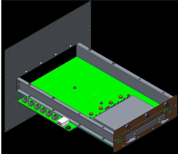
Figure [138437](#): LFF Card Thermal Test Fixture PCB
