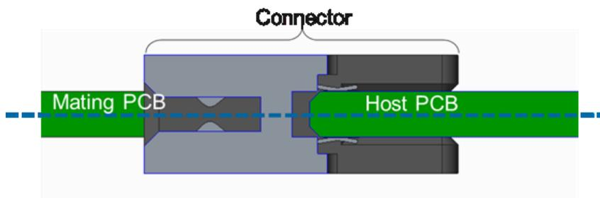
Figure 79: 0.3 mm Offset for 0.076" Thick Baseboards
