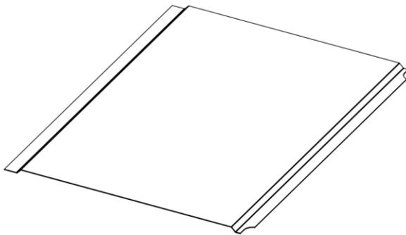
Figure 38: LFF Bottom Side Insulator (Top and Side View)
