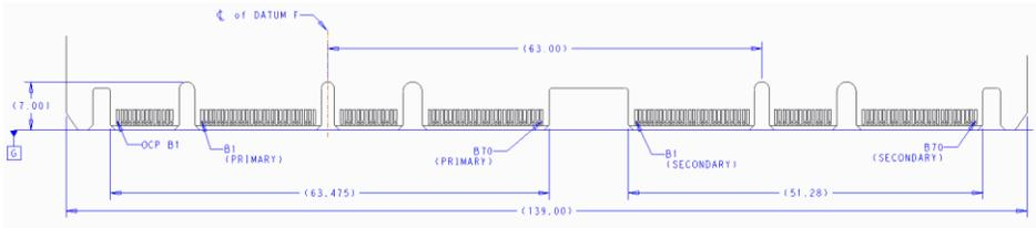
Figure 71: LFF Gold Finger Dimensions – x32 – Bottom Side (“A” Pins)
