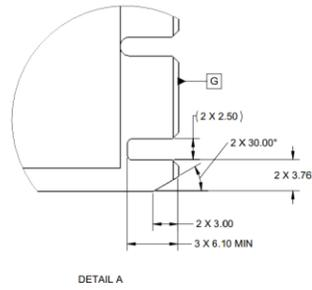
Figure 31: LFF Keep Out Zone – Bottom View
