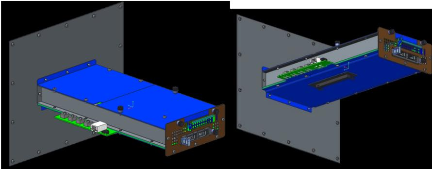
Figure 134133: SFF Thermal Test Fixture Preliminary Design – Cover Removed
