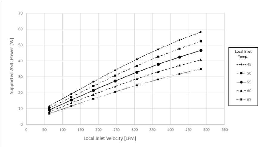
The curves shown in Figure 124Figure 123 were obtained using CFD analysis of the reference OCP NIC 3.0 LFF card. The reference card has a 45 mm x 45 mm ASIC with two QSFP connectors. Additional card geometry parameters and boundary conditions used in the reference CFD analysis are summarized in Table 66Table 65. Figure 125Figure 124 shows a comparison of the 3D CAD and CFD model geometry for the reference OCP NIC 3.0 card.
