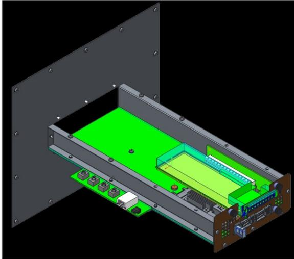
Figure 135134: SFF Card Thermal Test Fixture PCB
