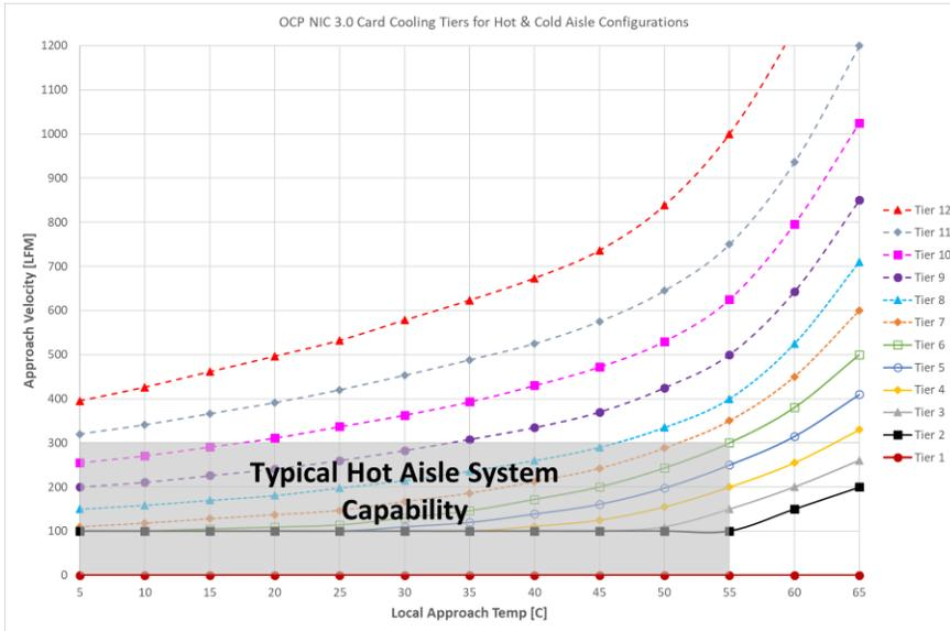
Figure 144143: Typical Operating Range for Cold Aisle Configurations
