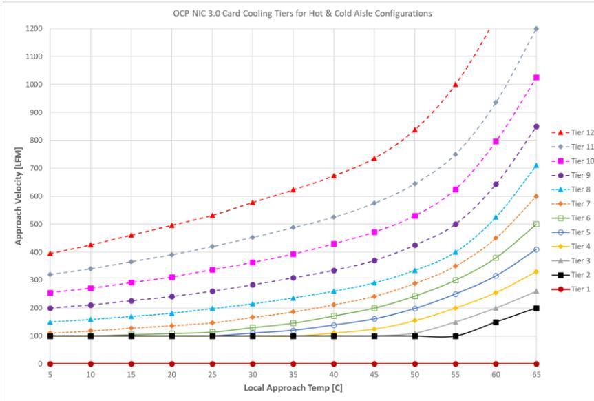
Figure 143142: Typical Operating Range for Hot Aisle Configurations
