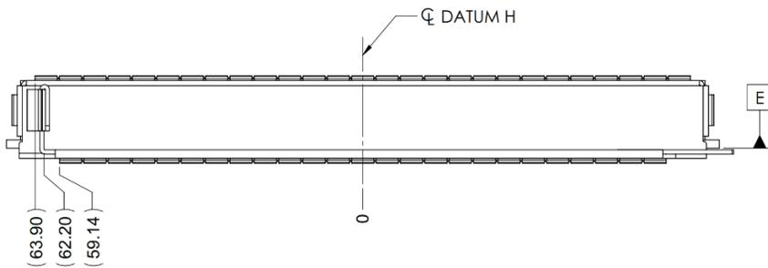
Figure 56: LFF OCP NIC 3.0 Card with Ejector CTF Dimensions (Side View)
