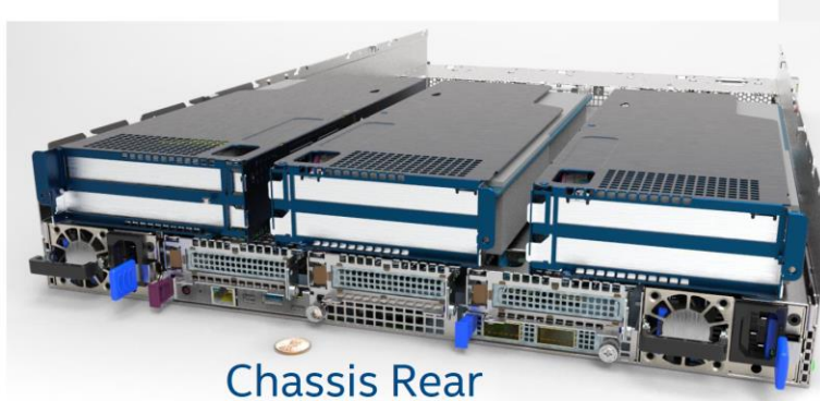
Figure 38. Typical 1U and 2U PCIe Slot Configurations for Rear Management System
