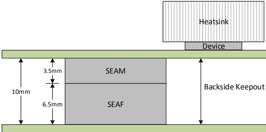
Figure 2. Connector stackup
