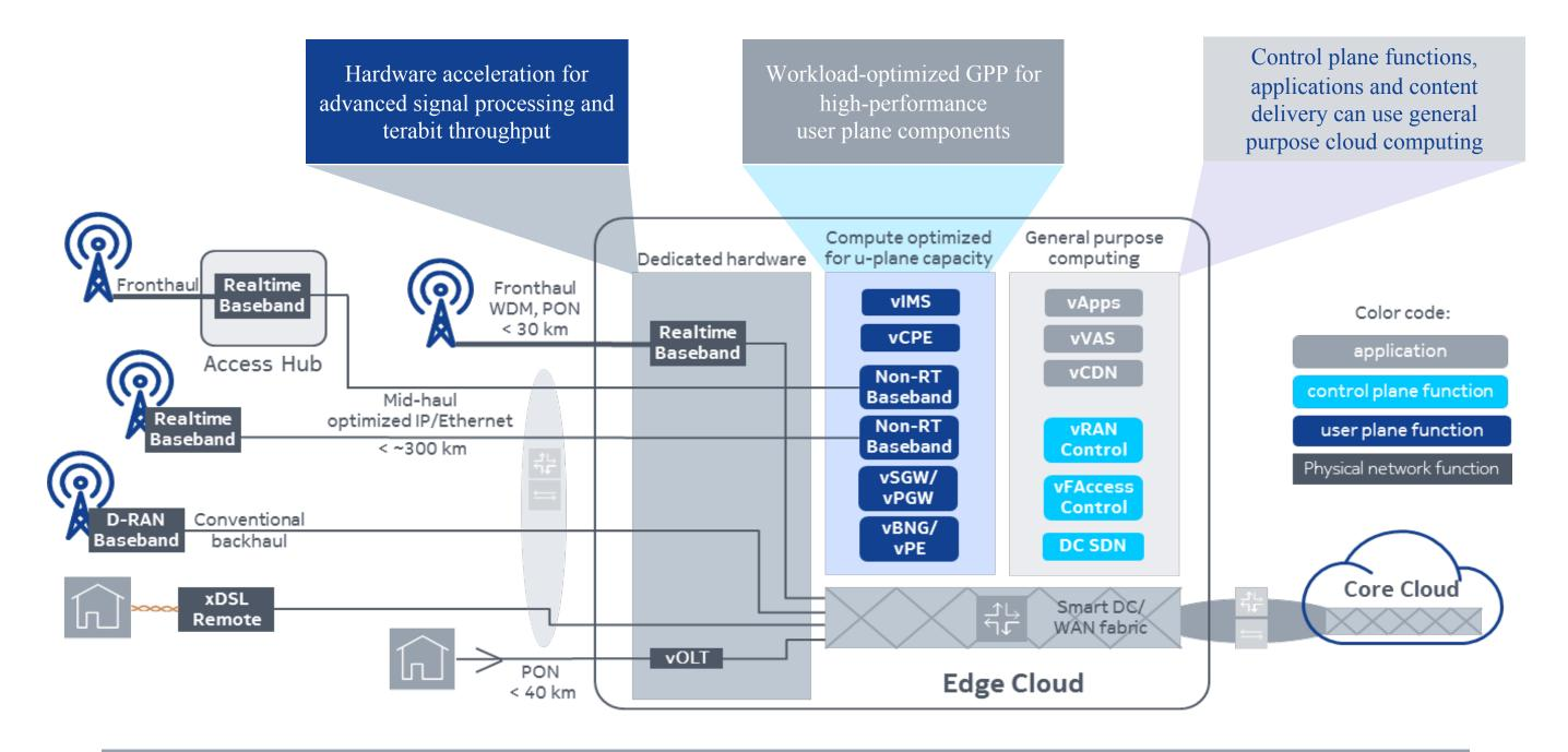
A target architecture for the Edge Cloud Data Center, all fiber in, all fiber out, converged across residential and enterprise, fixed and mobile.
