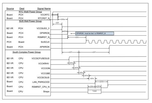
Power Sequencing Diagram G3 with RTC loss to S5
