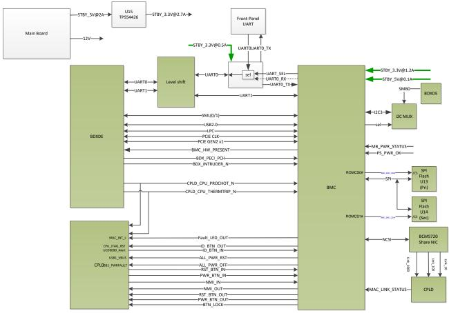
The following brief descriptions are for the interface between BMC module and CPU board in following sections.
