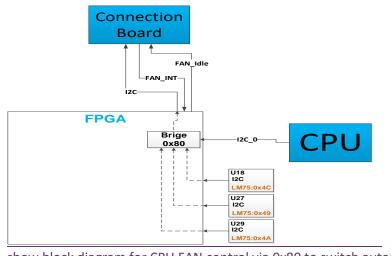
show block diagram for CPU FAN control via 0x80 to switch automatic or manual.
