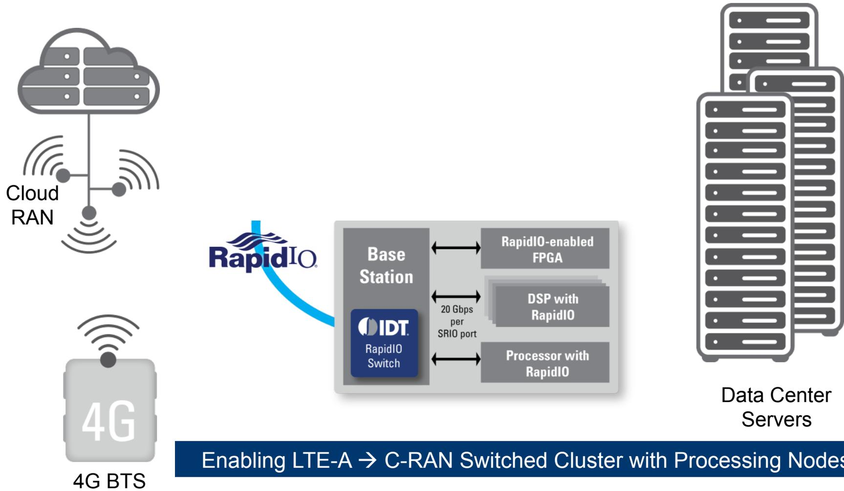
Enabling LTE-A → C-RAN Switched Cluster with Processing Nodes
