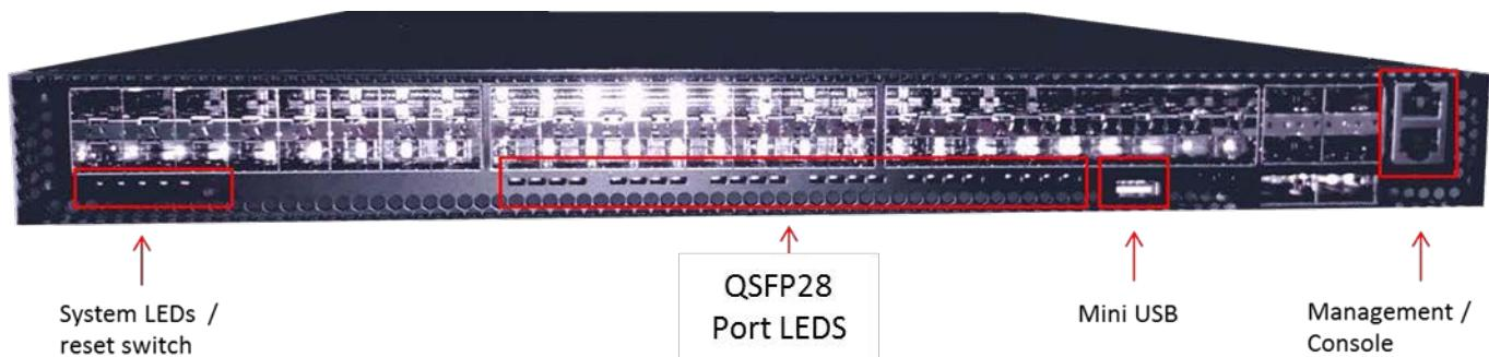
The front panel view of the AS5900-54X includes the following key components:
